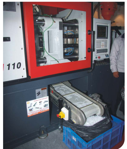
▲ Conveyor belt under Injection Moulding Inline Small Conveyor Belt to transfer multi cavity parts to prevent damage.
