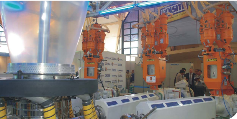
▲ Material Mixing & GSM Control: Online EPC – Gravimetric GSM Control System automate material conveying, feeding and controlling in one go with unique user-friendly touch screen. Each layer throughput is precisely monitored and controlled.
