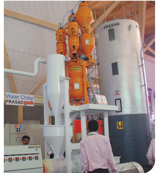
▲ Installation with tape plant: Multi component gravimetric dosing & mixing system ensure very accurate & consistent feeding of all materials. Central screw chiller circulate chilled water to entire plant & help to maintain quality & output of tapes. Prasad silo and silo feeding system save space, eliminate labour and contamination as well as control inventory.
