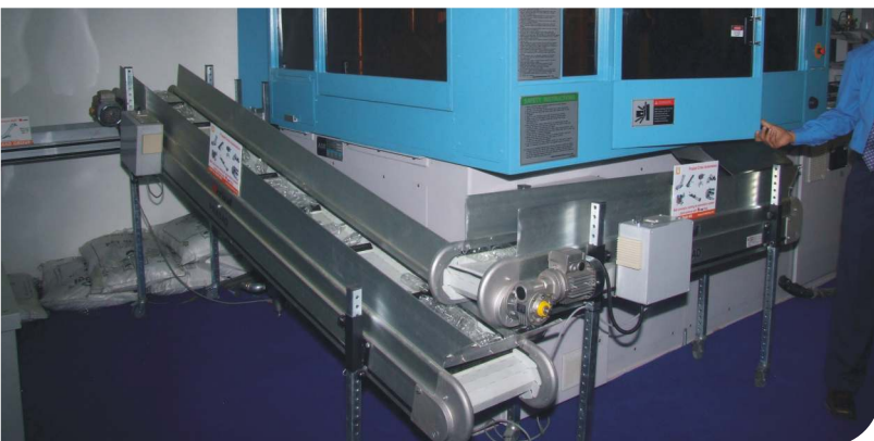
▲ Conveyor belt under ISBM This parts conveying system is completely untouched by humans and transfer bottles to packing area. It also fulfill clean room condition.
