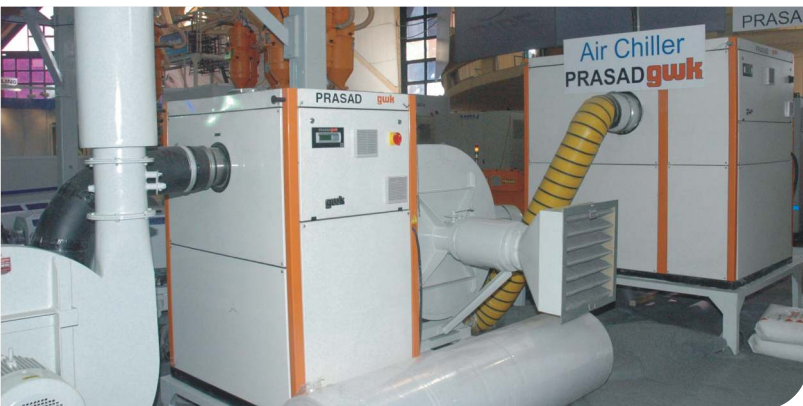
▲ Direct Air Chillers for blown film plant, gives uniform air temperature through out the day & lower air temperature at reduce power cost.
