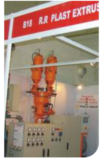
▲ Gravimetric Dosing Mixing System for drip line extruder for very accurate and consistent feeding of all materials
