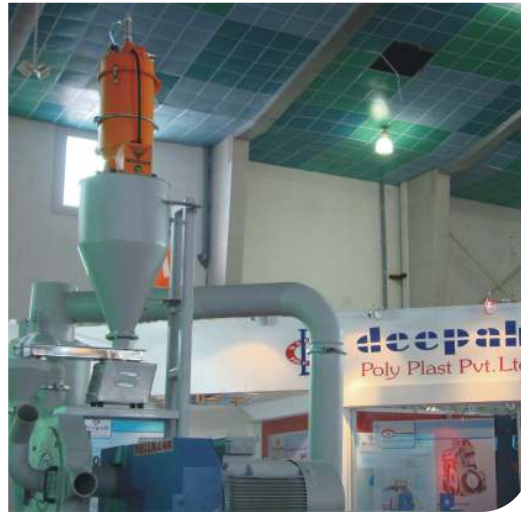
▲ Hopper Loader on high output pulveriser for maximum efficiency.
