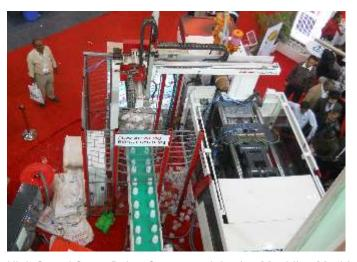
High Speed Servo Robot System on Injection Moulding Machine with Conveyor Belt and Safety Cage
