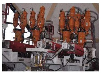
Multi Component Gravimetric Dosing Mixing System on Multi Layer Lamination Plant
