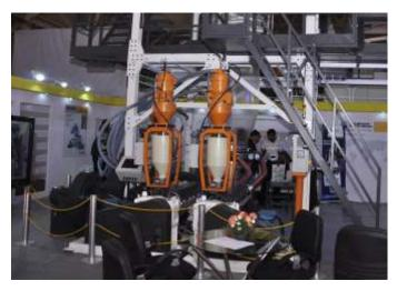
Extrusion Process Monitoring System on Three Layer Blown Film Plant for continuous display of output in each layer.
